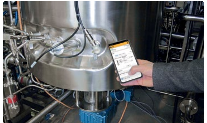
Figure 4. DO and pH sensors are often inserted in the side of production-scale bioreactors.
